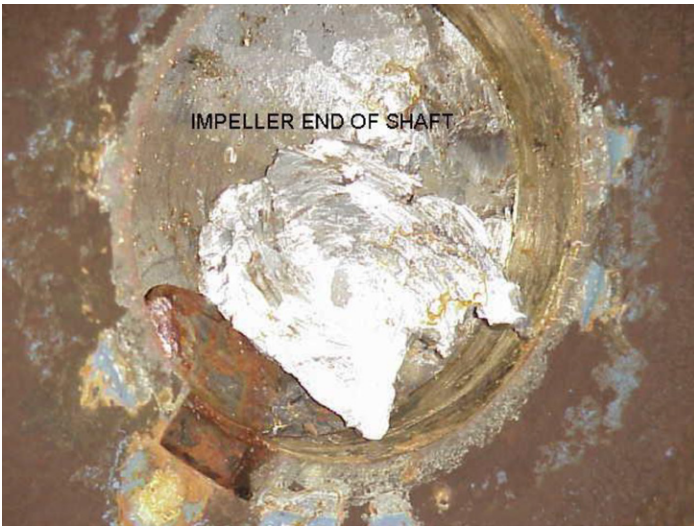
Figure 8 – Broken shaft at impeller end
