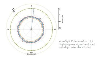
Software dual-tasking - The VibroSight software with the latest Hydro air-gap monitoring package support simultaneous data logging and data display. So for instance, you can display live data during a machine transient while the data is being stored in the database repository (historical data).
